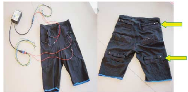
Figure 1 ES-shorts connected with the eight-channel Neuropro stimulator; front and back. Arrows indicate the electrodes for right g+h muscles.
