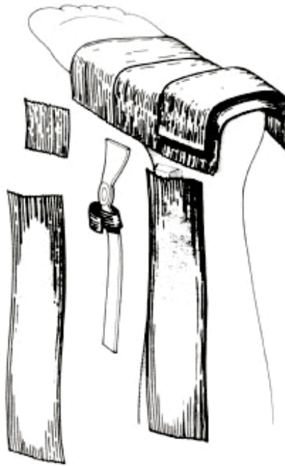
Figure 5. Exploded view of carbon tape and joint lay-up on a modified cast prior to trim.
