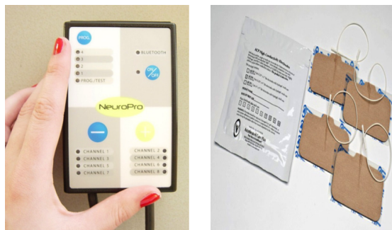
Figure 3. NeuroPro 8-channel electro stimulator, Axiobionics, Ann Arbor, MI, USA, with self-adhesive surface electrodes
