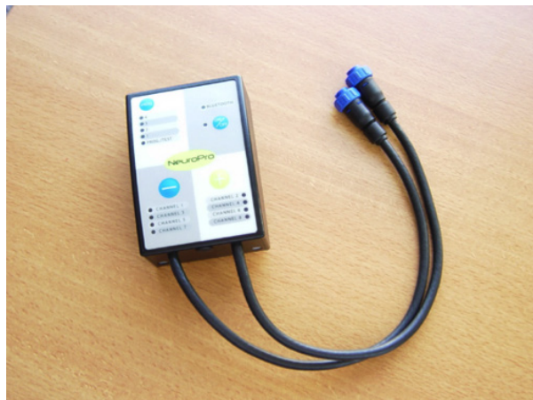
Neuropro 8-channel electrical stimulator. Suitable for research purposes, but not less user friendly for daily (clinical) use.
